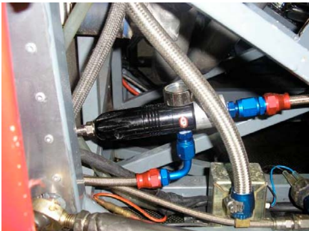
LP regulator to reduce 350psi feed from paintball cylinder Lower line goes to blipper. Right line to actuator.
